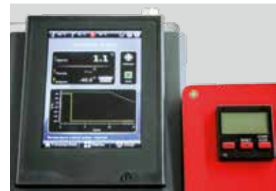
Temperature control touchscreen and timer display
