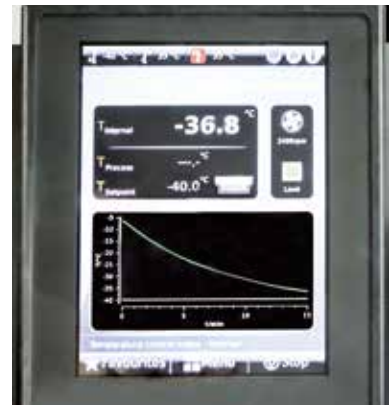
Sample temperature recording by optional immersion probe
