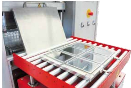
Six cavity sheet mould (6x 150x80x2mm)
