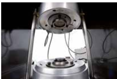
Die upgrades including precision heaters and probes
