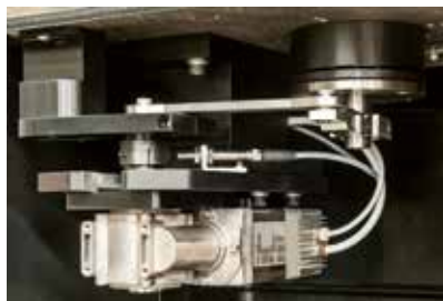
Rheometer brushless DC drive upgrade
