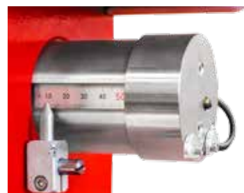
Anvil plate with integrated sample sensor and sample height adjustment
