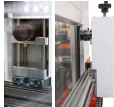
CCD Camera system for crack-growth measurement
